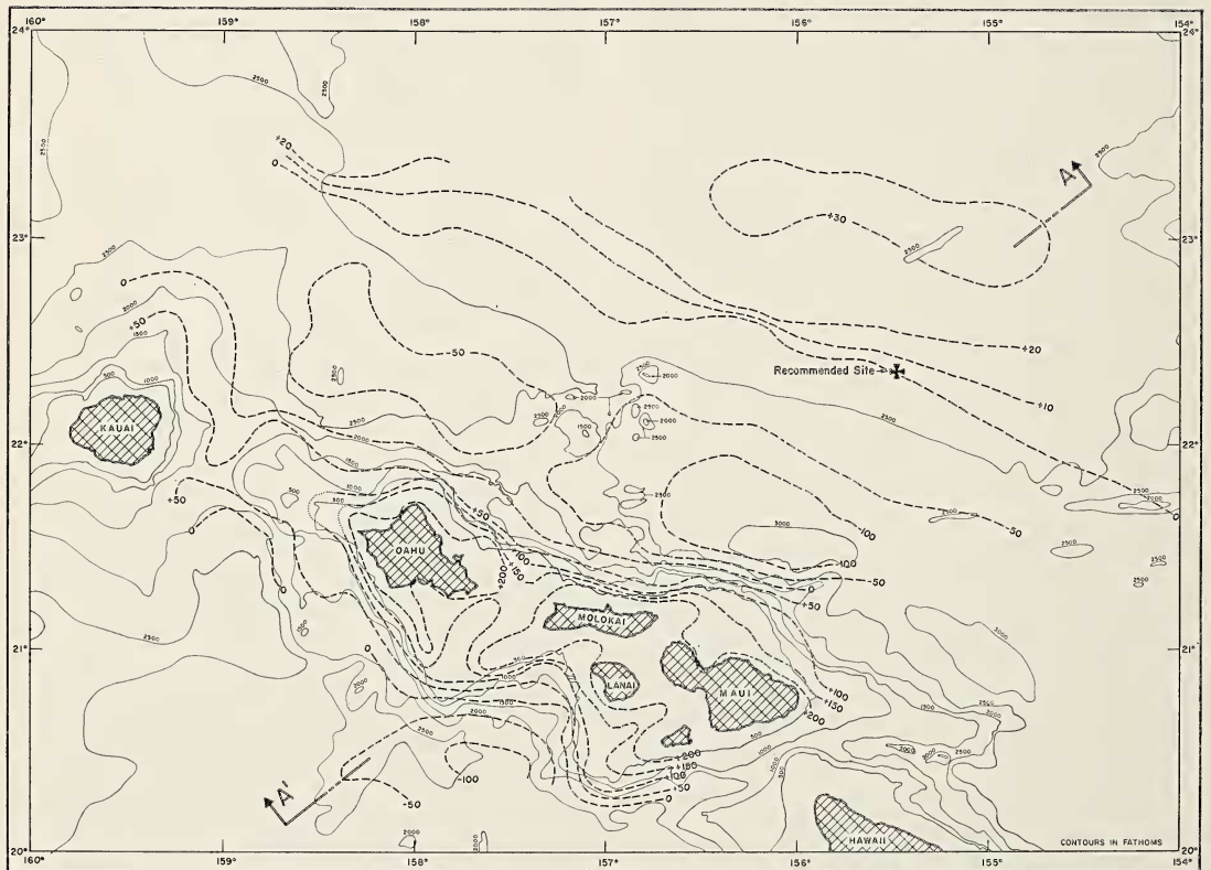
FIG. 3. Free air anomaly ( dashed lines ) gravity map of the Hawaiian Islands (values in milligals). Bathymetry contours ( solid lines ) in fathoms.
